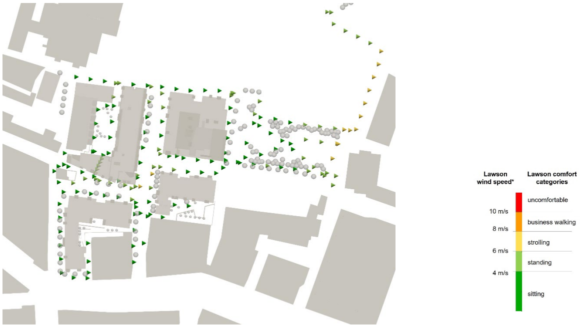
Figure 39. Lawson wind speeds at key locations along the thoroughfares of the proposed development in existing surroundings with landscaping
