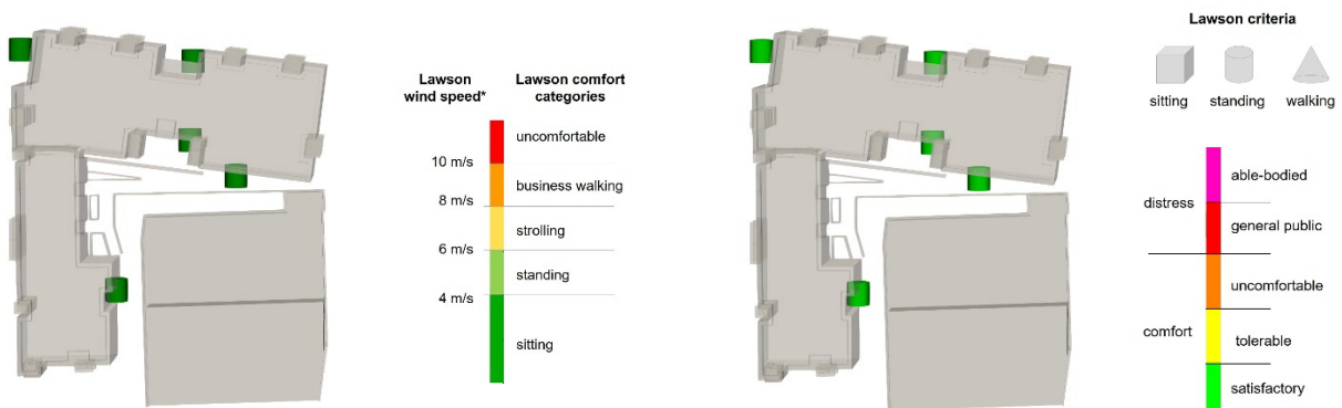
Figure 32: Lawson wind speeds (left) and Lawson criteria (right) at the primary entrances of BG4
