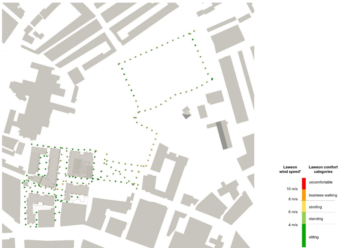
Figure 9: Overview of the Lawson wind speeds at key locations along the thoroughfares around the site in existing surroundings
