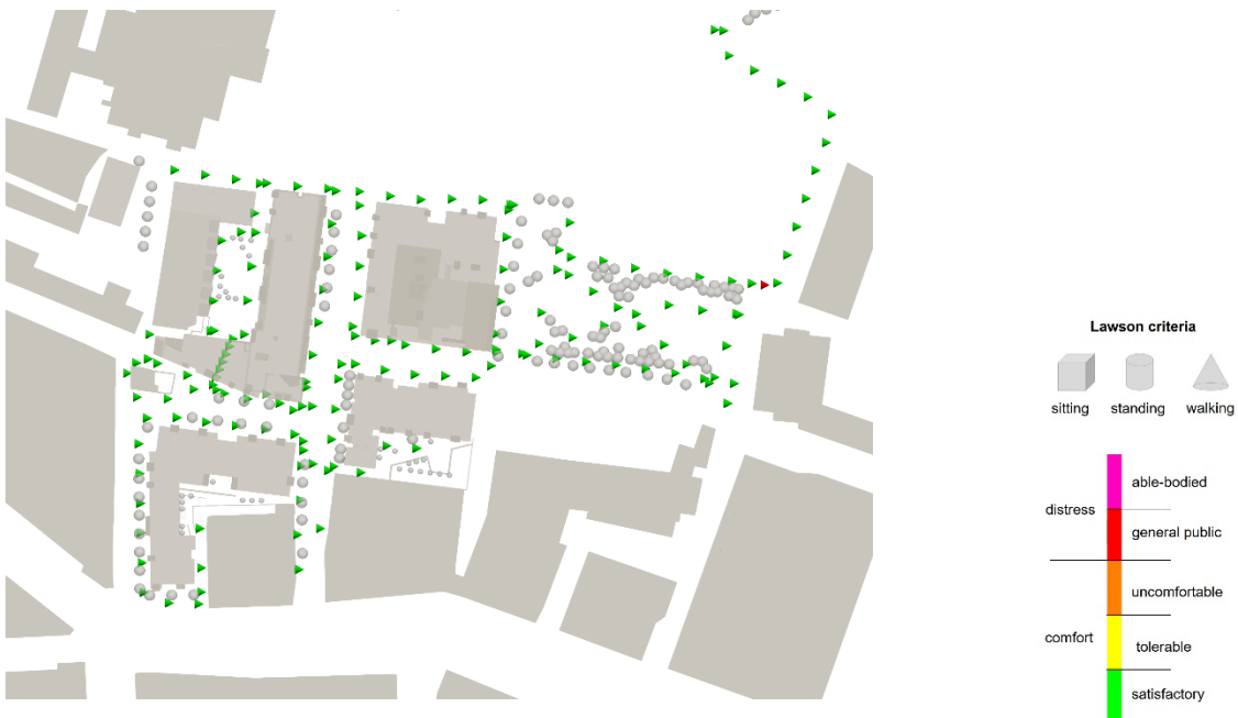
Figure 40: Lawson criteria at key locations along the thoroughfares of the proposed development in existing surroundings with landscaping
