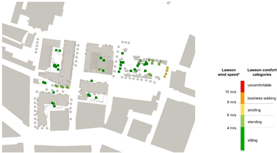
Figure 41. Lawson wind speeds at key locations of the public open spaces within the proposed development in existing surroundings with landscaping
