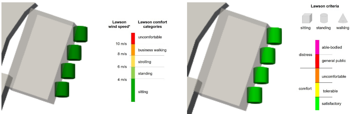
Figure 37: Lawson wind speeds (left) and Lawson criteria (right) at the primary entrances of BG5
