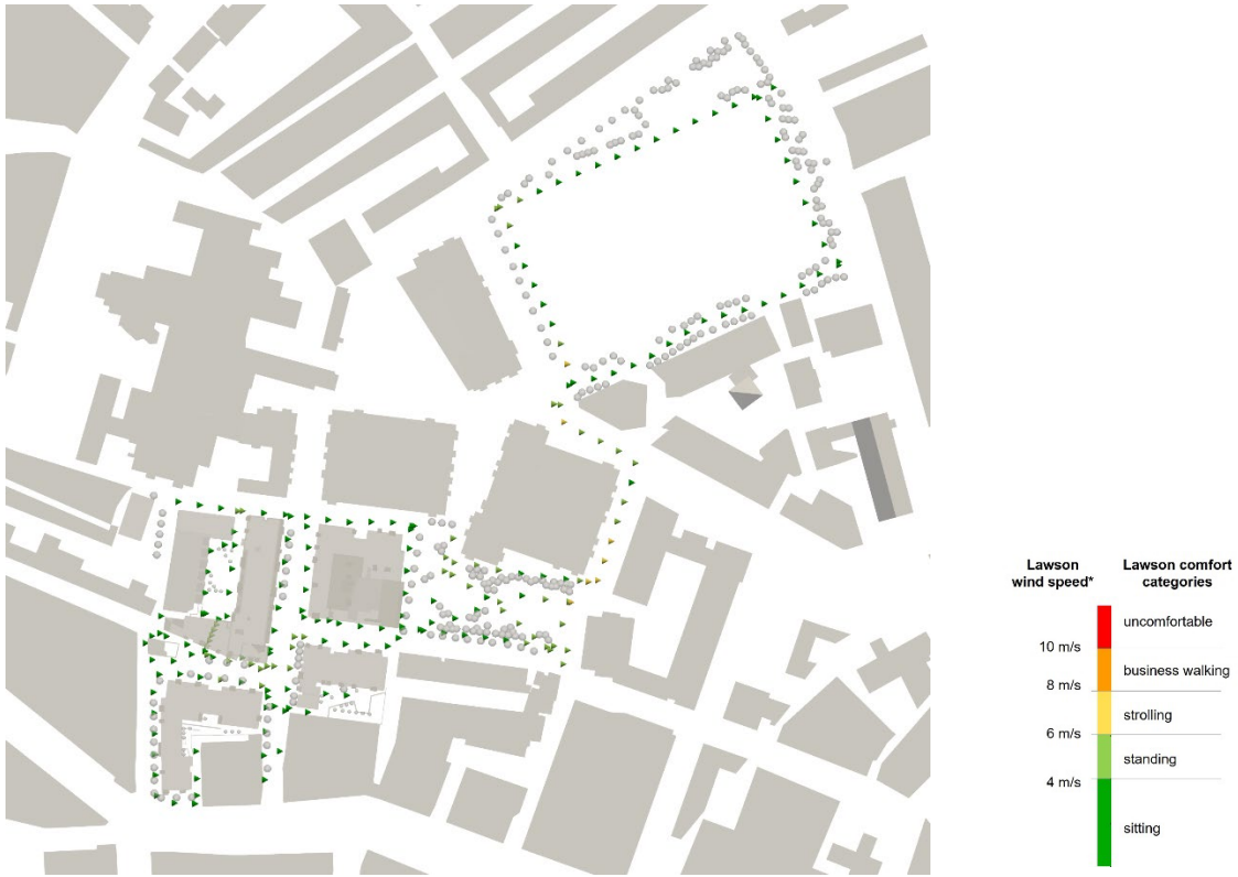
Figure 44: Overview of the Lawson wind speeds at key locations along the thoroughfares around the site in cumulative (future) surroundings with landscaping
