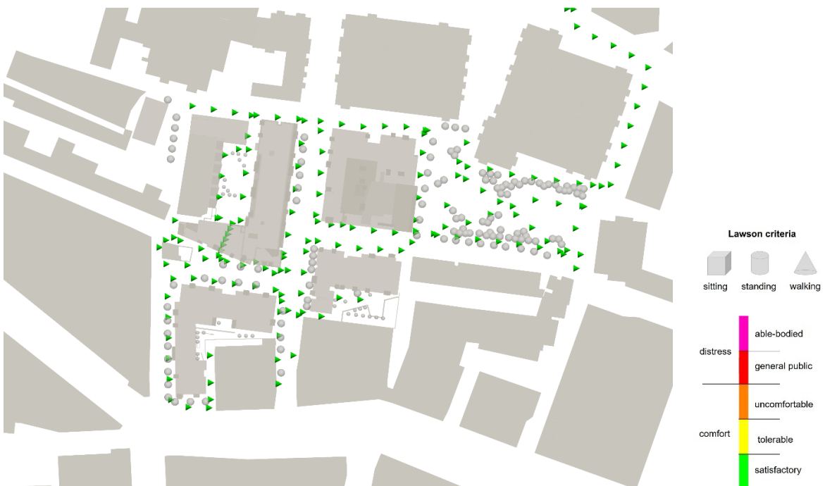
Figure 45: Lawson criteria at key locations along the thoroughfares of the proposed development in future surroundings with landscaping
