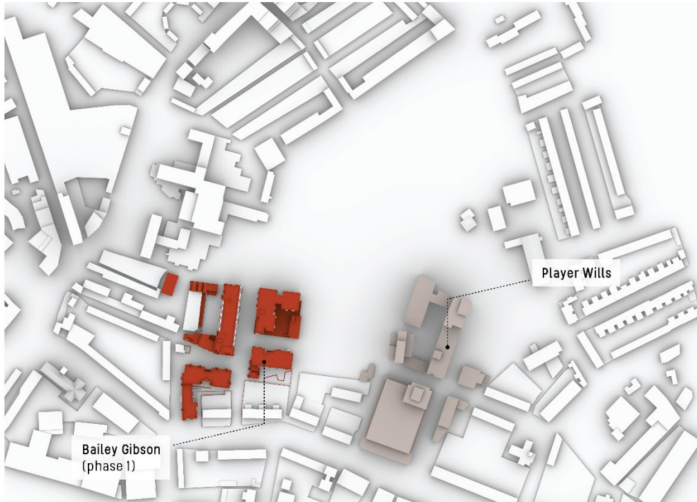
Figure 7: Top view of the proposed development and the existing surroundings as represented in the CFD model
