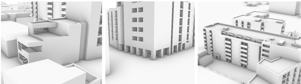
Figure 8: Examples of design features of Block BG1 that have a positive impact on the wind conditions: Slatted screens (left), recessed building entrance (centre), canopies and side screens on the rooftop terraces (right) BG1
