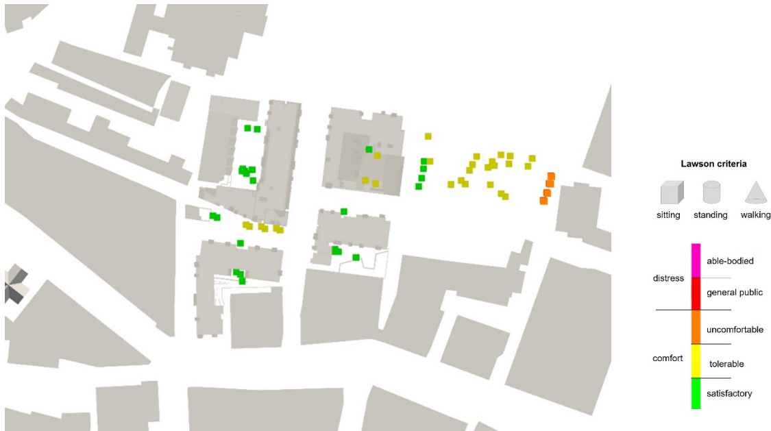
Figure 14: Lawson criteria at key locations of the public open spaces within the proposed development in existing surroundings
