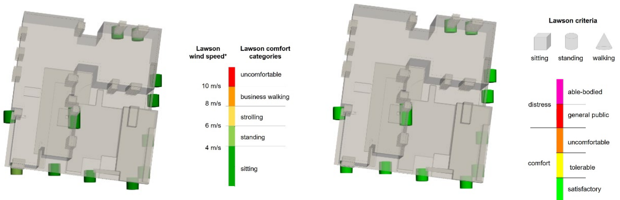
Figure 21: Lawson wind speeds (left) and Lawson criteria (right) at the primary entrances of BG2
