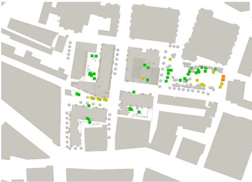
Figure 47: Lawson criteria at key locations of the public open spaces within the proposed development in future surroundings with landscaping
