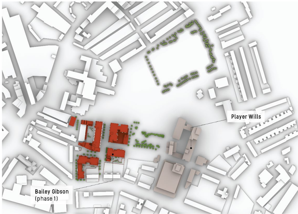
Figure 38: Top view of the proposed development with landscaping and the existing surroundings as represented in the CFD model
