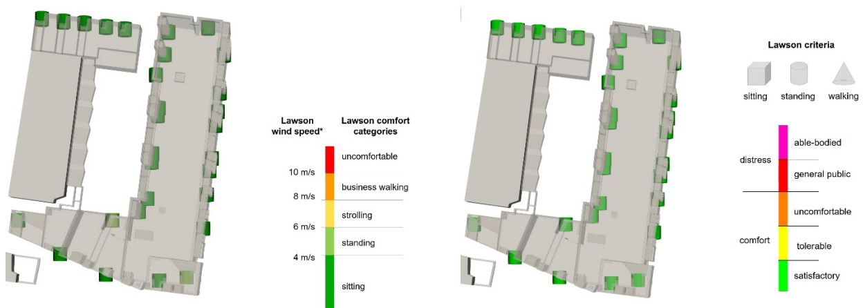
Figure 15: Lawson wind speeds (left) and Lawson criteria (right) at the primary entrances of BG1
