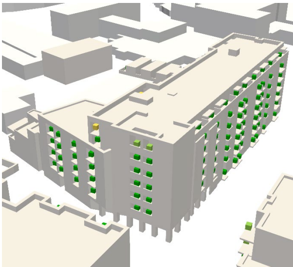
Figure 16: Lawson wind speeds at BG1 balconies of the proposed development in existing surroundings (SE view)
